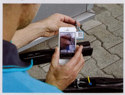
Technician installing an eMitter Indoor Rocker by scanning the QR-Code with the App. The device is then placed in a Runbox Robust tunnel station, equipped with two Gorilla Traps for mice and will alert the technician via the app as soon as a trap is triggered. The Runbox Robust is very durable and can be used in wet areas. The material is insulating and creates warm and comfortable conditions which are attractive to mice. Photo: Futura
